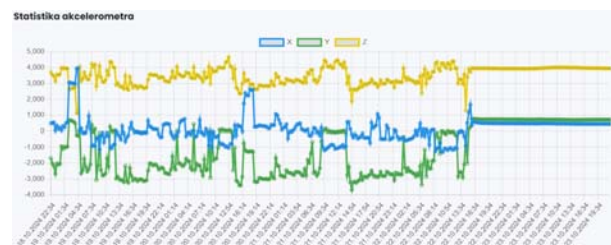
Fig. 7. Current acceleration of the device during observation period.
